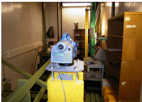
Fig. 3. The FGI system calibration in the FGI laboratory (left). Especially designed for the Zeiss DiNi12 digital levelling system with two observation pillars.
